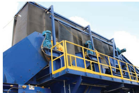
Drum Magnet Feeder GK's Two-Mass Vibratory Feeders dynamically compensate for surge loadings to provide uniform feed to the drum magnet.
