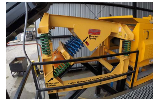
High Stroke Feeder Dynamic response to load surges, increased feed capacity, exceptional reliability, and ease of maintainability. High Stroke Feeders are specifically designed to enhance your process.
