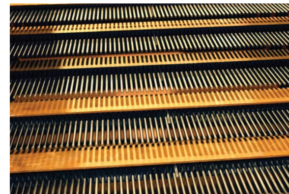
Rod Deck Screen Designed for separation of difficult material that is prone to sticking or blinding in traditional screening applications using the flexibility of the individual rods within the deck section.
