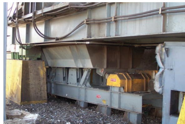
Under Mill Oscillator Designed with extra structural and gridwork reinforcement to ensure trough integrity that will withstand the severe conditions found underneath auto-shredders.
